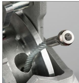
*LUG-ALL Exclusive: Other brands use set screws requiring 2 to 3 unusable wraps of cable around the drum. Our unique ball-shank-terminal securely anchors the cable to its drum, so you get full use of your cable length!*
