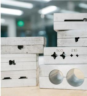
Round, square and X profiles standard, custom profile molds created on demand with no tooling charges.
