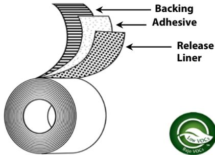
**Backing:** Printed 2.1 mil Aluminum Foil
