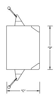
ETL Listed Conforms to UL Std. 514C 2-HR Fire Wall Rating ETL Control # 3107144 Suitable for Masonry Walls Material is Rigid PVC All dimensions are nominal See NEC Article 314 for use
