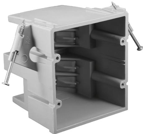
EZ35DN-HW is a 2-gang 35 cu. in. heavy wall residential EZ BOX that is ideal for new work applications for residential and light commercial projects where an even more durable box is preferred. The harder shell is designed to resist flexing and hold its shape in extreme conditions. It also features enhanced angled nails for easy mounting between studs 8 wire clamps for EZ and secure wiring.
