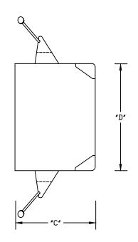
ETL Listed Conforms to UL Std. 514C 2-HR Fire Wall Rating ETL Control # 3107144 Suitable for Masonry Walls Material is Rigid PVC All dimensions are nominal See NEC Article 314 for use
