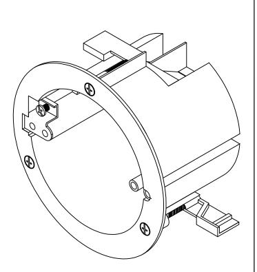
UL Listed UL File # R18795 and E98429 2 Hour Ceiling Fire Rated Material is Polycarbonate UL Category Codes CEYY, QBWY and QCMZ 18 Cubic Inches Volume Fixture Weight is 6 lbs Maximum Ground Lug included
