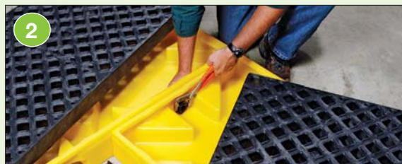
Next, connect the decks with the Bulkhead Fittings.
