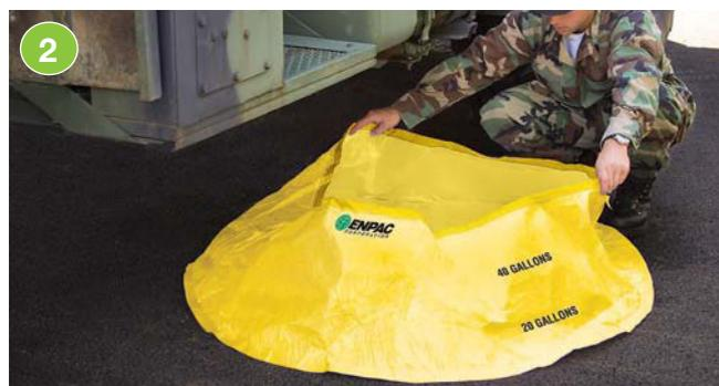
Step 2: Position pool underneath spill source.
