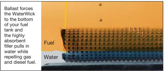
Ballast forces the WaterWick to the bottom of your fuel tank and the highly absorbent filler pulls in water while repelling gas and diesel fuel.
