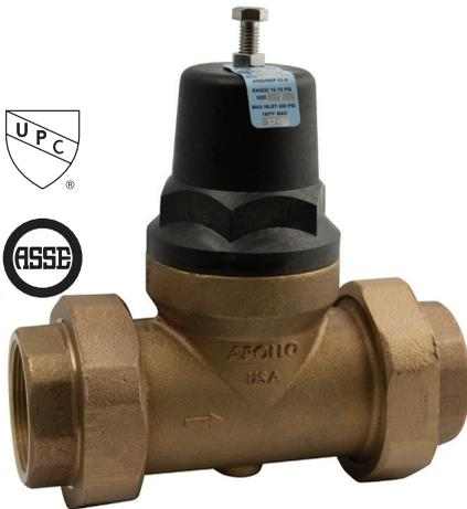
The new large diameter Apollo<sup>®</sup> Lead Free Pressure Reducing Valve Model PRE (36ELF Series) is designed to conserve water and protect water distribution systems by automatically reducing elevated supply pressures. The dezincification resistant bronze body, stainless steel adjusting screw and dielectric polymer cage provide maximum corrosion resistance. Designed for easy in-line servicing with simple cartridge removal.
