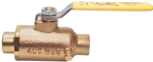
Perfect choice for hydronic and water systems where system draining is required. Replaces globe style stop and waste valves. Designed to be soft soldered into lines with no disassembly.
