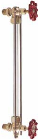
Use for all types of liquid level verification; available with 3/8" or 1/2" NPT male pipe connections. Aluminum or plastic composition hand wheels; EPDM gauge glass gaskets standard. Other glass gaskets available.
