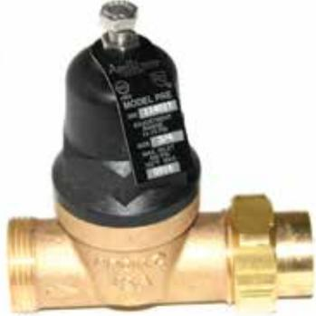
Designed for light duty residential and commercial applications to protect water supplies from excessive pressure. Excellent flow performance at low pressure drop. The dezincification resistant bronze body and dielectric polymer cage provide maximum corrosion resistance. Designed for easy in-line servicing with simple cartridge removal. They meet ASSE 1003 and CSA B356 standards. They are listed with IAPMO and the city of Los Angeles.
