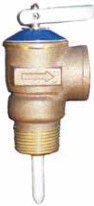
Automatic temperature and pressure relief valves feature unique non-metallic coating which protects the element against galvanic and electromechanical corrosion by isolating it from the heated water. This coating is electrostatically applied for uniform coverage, then thermobonded, resulting in optimum adhesion for extended service life. **CSA** design certified at all settings to ANSI Z21.22. **ASME Section IV** rated at 125 psig and 150 psig settings for 3/4" NPT only.
