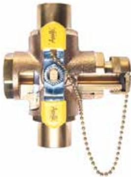
Straight-through flow; all brass cover and chain prevent accidental system drainage; hose thread connection for disposal of drained media.
