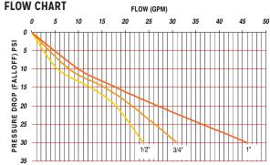
ote: Flow curves are based on static conditions of 100psi inlet pressure and 50 psi outlet pressure. Pressure differential is the difference between the supply pressure and adjusted outlet pressure measured in the static (closed) condition. Pressure fall-off is the decrease in downstream regulated pressure as the flow increases.
