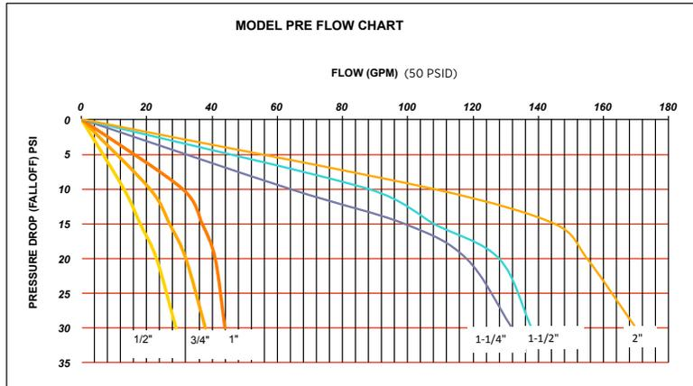
*Pressure Differential is the difference between the inlet supply pressure and the adjusted outlet pressure.*
