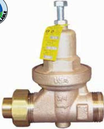
Apollo PR Series pressure reducing valves provide automatic control of excessive water pressure and problem supply fluctuations. These models are designed to reduce pressures of up to 300 PSI to a more manageable range.
