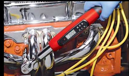
Multiple Alerts when the desired torque setting is reached prevent over-torquing of bolts.
