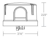
The DP Series photocontrols utilize premium components and silicon light sensors which resist long-term drift of the turn-on level. This series includes the utility-preferred 1704 and 1707 costeffective, but extremely robust, control for non-LED fixtures.
