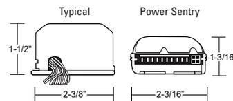
New reduced-profile design fits in the tightest of applications
