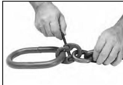
2. Place stud assembly and alloy locking pin in link as shown.
