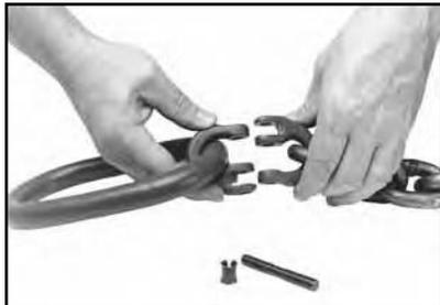
1. Loop one half of body over the master link at the flat embossed area, the other half through the chain. Fit together.
