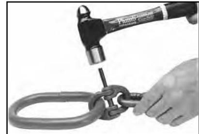
3. Drive the locking pin in until the snap ring engages the recessed portion of the pin. (Link is disassembled by simply driving locking pin out.)
