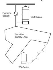
Well-X-Trol 440 through 460 Series are sometimes used on pressure regulation stations to provide system dampening during periodic high peak loading such as laundry wheels.
