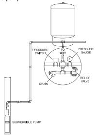
2. In a municipal well system or pressure boosting station, Well-X-Trol's are used to control sequential start of the main pumps. At the same time, it reduces surge and provides the jockey pump with guaranteed minimum run times during low peak demand periods.
