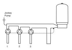
**4.** Well-X-Trol 400 Series are also used for high pressure booster applications, e.g. high rise buildings, irrigation systems and community wells.
