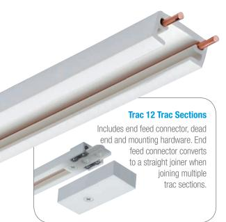
Trac 12 is the original miniature, low voltage system that combines a 20-amp capacity with an extremely small, engineered-plastic profile. The system operates using remotely located or in-line 2-volt or 24-volt transformers. A maximum of 240 watts (12 volts) or 480 watts (24 volts) can be placed per circuit of trac.
