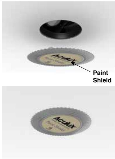
**Step 5.** Peel off 3M™ adhesive release liner, line-up parts (per step 4), and firmly press flush mount adapter onto drywall. Hold for at least 5 seconds for a bond to develop. *Do not remove the paint shield.*
