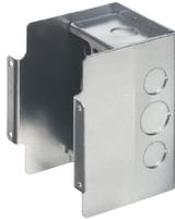
Recessed, metallic electrical box with non-metallic, extra-duty weatherproof-in-use cover for flat surfaces in existing construction. Accepts most single gang wiring devices and uses standard indoor wall plates or a GFCI cover plate. Non-metallic portion and covers are UV rated plastic for long outdoor life.
