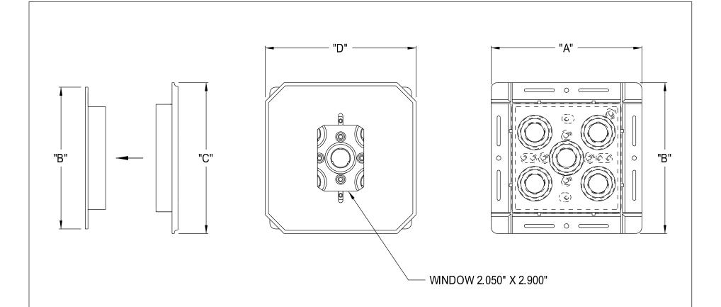
THIS STYLE HAS IMPRESSIONS ON THE BACK SIDE. BY SIMPLY CUTTING ALONG THE IMPRESSIONS AND REMOVING MATERIAL, THIS BLOCK CAN BE USED FOR 4" ROUND OR 3 1/4" ROUND CONFIGURATIONS.
