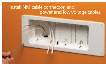
**3** Mount box (horizontal) between 16" o.c. studs through remaining (4) holes in trim plate. Use (4) #8 x 1-1/2" (supplied) screws.
