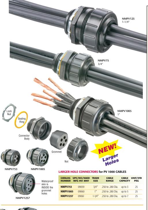
Arlington's UV rated, multi-hole connectors are ideal for solar and other outdoor jobs requiring the connection of multiple cables into raceways, fittings, and combiner or junction boxes.
