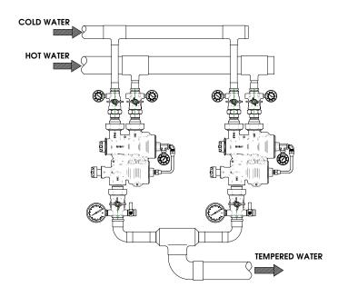
SUGGESTED INSTALLATION FOR HIGH FLOW PARALLEL CONNECTION
