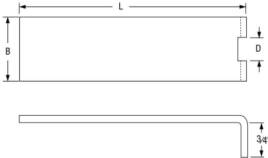
**FIG. 89: RETAINING CLIP: DIMENSIONS (IN) • WEIGHT (LBS)**
