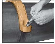
**BOLTS**— Apply a thin coat of Xtreme lube to the bolt threads. Tighten the nuts alternately and equally to the specified bolt torque.
