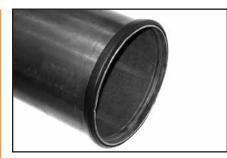
**2 GASKET INSTALLATION**— Slip the gasket over the pipe end, making sure the gasket lip does not overhang the pipe end.
