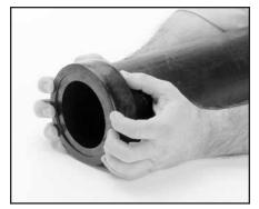
**3 GASKET INSTALLATION**—Slip the gasket over one of the pipe ends. Make sure the gasket does not overhang the pipe end. Align the second pipe and while holding it in the butted position, slide the gasket back over the second pipe end. The gasket must be positioned on the gasket seat surface of the grooved steel pipe. Make sure the gasket does not overhang into the pipe groove.
