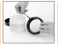
2CHECK & LUBRICATE GASKET— Check to assure the gasket material is acceptable for the intended service. The Gasket color code is green for EPDM and orange for Nitrile (Buna-N).
