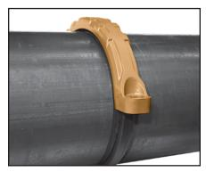
HOUSING— Place each housing half on the pipe and into each groove making sure that the gasket does not slip out of position in between the pipe ends or groove.
