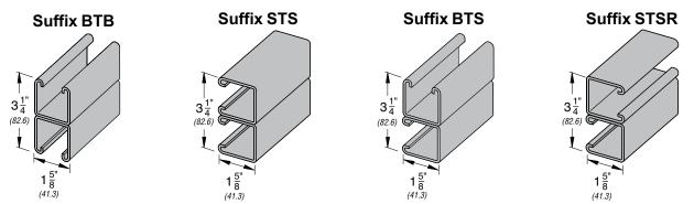
Our welded channels are spot welded 2" (50.8mm) on center, dimensions shown are for welded variations of any channel with or without slotted holes.
