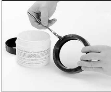
**2 CHECK & LUBRICATE GASKET**— Check to assure the gasket material is acceptable for the intended service. The Gasket color code is green for EPDM and orange for Nitrile (Buna-N).
