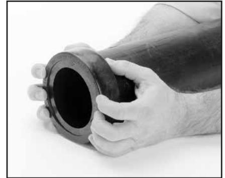
**3 GASKET INSTALLATION**— Slip the gasket over one of the pipe ends. Make sure the gasket does not overhang the pipe end. Align the second pipe and while holding it in the butted position, slide the gasket back over the second pipe end. The gasket must be positioned on the gasket seat surface of the grooved steel pipe. Make sure the gasket does not overhang into the pipe groove.
