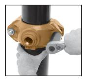
**TIGHTEN NUTS**— Re-insert the bolt and run-up both nuts finger tight. Securely tighten the nuts alternately and equally until they are completely tightened and there is no gap between the bolt pads. Continue tightening the nuts alternately and equally until the specified bolt torque is reached.
