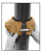
HOUSING ASSEMBLY— With one nut and bolt removed and the other loosened. place one side of the housing over the gasket. Make sure the ribs on the outside of the gasket align with the recesses in the housing and the keys in the housing are in the grooves on both pipes. Swing the other housing over the gasket and into the grooves on both sides of the pipe. Make sure the recess in the outlet of the housing is properly aligned with gasket outlet.
