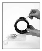
**CHECK & LUBRICATE** GASKET— Check gasket to be sure it is compatible for the intended service. Apply a thin coating of Gruvlok lubricant to the exterior surface and sealing lips of the gasket. Be careful that foreign particles do not adhere to lubricated surfaces.
