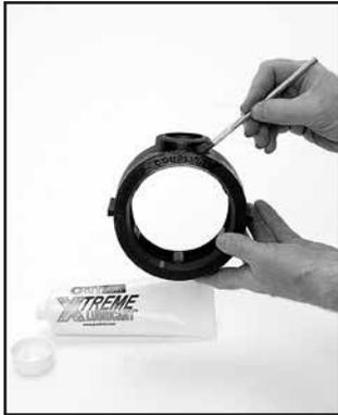
**1 CHECK & LUBRICATE GASKET**— Check gasket to be sure it is compatible for the intended service. Apply a thin coating of Gruvlok lubricant to the exterior surface and sealing lips of the gasket. Be careful that foreign particles do not adhere to lubricated surfaces.
