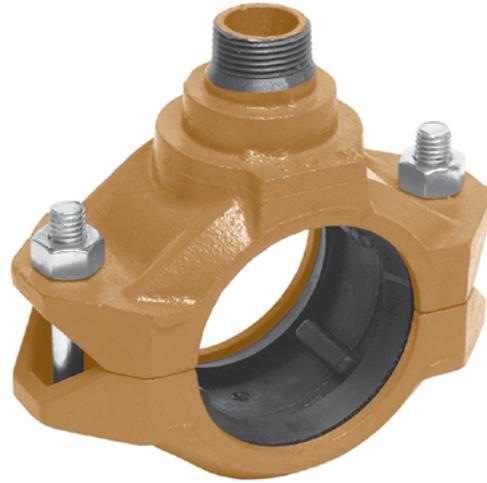
The Figure 7074 Cast Caps are **NOT** recommended for use on run connections. Contact an Anvil Representative for additional details. Figure 7075 Bull Plugs must be used on end of line run connections. Figure 7074 Cast Caps may be used on Figure 7042G outlet connections. Flow into the outlet connection of the Figure 7042 Outlet Couplings must not exceed 7 ft./sec.
