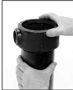
**2 GASKET INSTALLATION**— Slip the gasket over one pipe end making sure the pipe abuts the gasket's center ribs.
