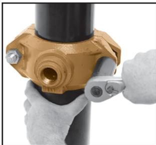
**5 TIGHTEN NUTS**— Re-insert the bolt and run-up both nuts finger tight. Securely tighten the nuts alternately and equally until they are completely tightened and there is no gap between the bolt pads. Continue tightening the nuts alternately and equally until the specified bolt torque is reached.
