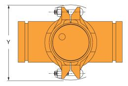
NOTE: The above illustration shows the required orientation of the Rigidlok access coupling for assembly with a grooved-end flange.
