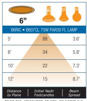
BEAM DIA. MEASURED AT 50% OF NADIR F.C.
