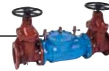
The DC100 provides protection against back-pressure and back-siphonage. The body and gate valves are constructed from epoxy coated ductile iron and corrosion resistant internal components. The DC100 is designed to streamline the number of working parts, making maintenance easy. The unique top-entry cover allows quick access to both check valves. The Double Check Backflow preventers are available in 2-1/2" thru 10" sizes. UL and FM approved.
