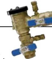
The PVB Pressure Vacuum Breaker is designed to be installed in high hazard service to provide protection against back-siphonage. It incorporates an independently acting check valve with a spring loaded float disc. When the internal pressure of the device falls to 1 psi or less, the float disc opens to atmosphere, preventing back-siphonage. Made with a bronze body and available in 3/4" thru 2" sizes.
