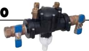
The Cash Acme RP500 does not contain lead or heavy metals and is no-lead compliant. The RP500 protects against high hazard backflow or back siphonage the valve is not susceptible to corrosion in aggressive water conditions and acts as a dielectric coupler in the water system. The unique top entry cover allows quick access to both check valves and relief valve. Available in 1/2" through 2" sizes, and comes standard with an air gap drain.
