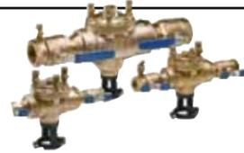
A Cash Acme RP100 or RP200 (Reduced Pressure Backflow Preventer) provides maximum protection against back-pressure and back-siphonage. The RP consists of two independently acting check valves and a relief valve. The Cash Acme RP100 and RP200 design streamlines the number of working parts, making maintenance easy. The unique top-entry cover allows quick access to both check valves and relief valve. The RP100 is available in 3/4" through 2" sizes and the RP200 comes in 1/2" and 3/4" sizes.
