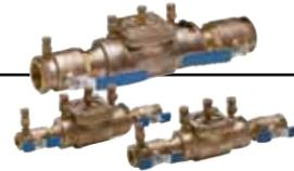
The DC100 provides protection against back-pressure and back-siphonage. The DC100 body and ball valves are constructed from bronze and corrosion resistant internal components. The DC100 design streamlines the number of working parts, making maintenance easy. The unique top-entry cover allows quick access to both check valves. The DC100 Double Check Backflow Preventers are available in 3/4" through 2" sizes.
