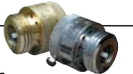
V-3 Backflow Preventers are for use around homes, schools, commercial buildings, laboratories and any place involving moveable hoses that are attached to threaded faucets. The Cash Acme V-3 attaches to any standard male 3/4" hose-thread sill cock. The valve is fitted with a male outlet connection to permit garden hose attachment.
