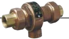
The BFP is designed for use at cross-connections when the danger from backflow does not present a health hazard. It is ideally suited for boiler feed lines, dairy processing systems, livestock drinking fountains, chlorinators, trap primers and numerous other similar applications. Available in a 1/2" size with threaded female union inlet and outlet connections and 1/2" threaded female drain connection.
