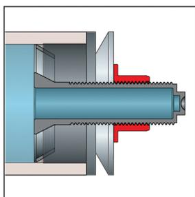
Hollow stem allows the system to be filled with water and provides a controlled drain down with a standard garden hose.
