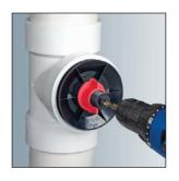
Use a 9/16" drill bit to open stem for use. A depression is furnished in the end of the stem to accommodate a drill bit.
