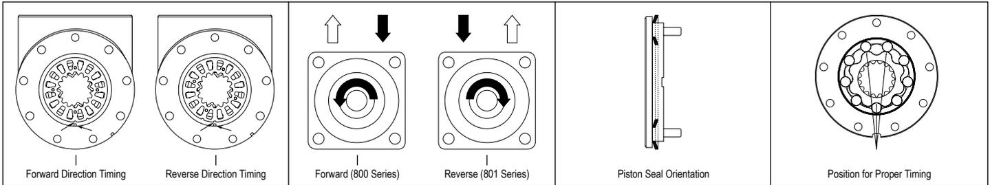
FIGURE 1 - Commutator Orientation
