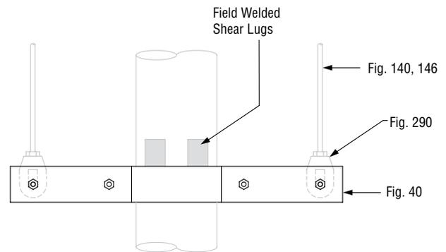
For Shear Lug Dimensions, refer to Special Design Products Fig. 40SD.
