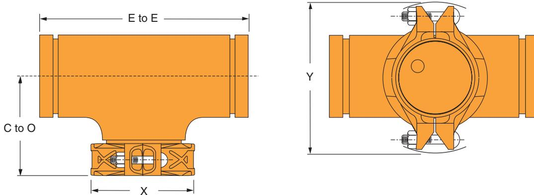
**NOTE:** The above illustration shows the required orientation of the Rigidlok access coupling for assembly with a grooved-end flange.
