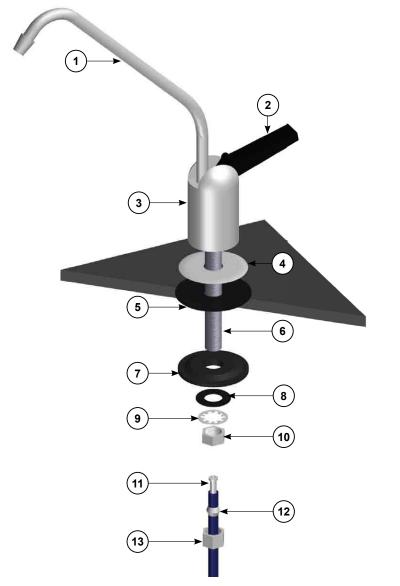
Figure A: List of Parts and Assembly in Exploded View
