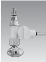
**Step B** – Connect the black tube from the RO module to the Adapt-A-Valve™ that is connected to the hot water angle stop valve. Leave enough tube so it is not kinked and cut the tube to the desired length.
