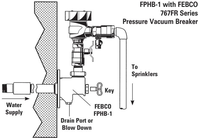
**Note:** PVB's must be installed a minimum of 12" above the highest point of water in the sprinkler system.
