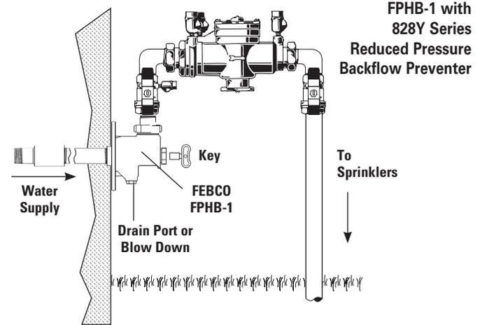
**Note:** RPZ's must be installed a minimum 12" above ground level.
