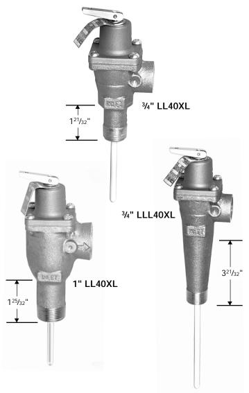
Following installation, the valve lever MUST be operated AT LEAST ONCE A YEAR by the water heater owner to ensure that the waterways are clear. Certain naturally occurring mineral deposits may adhere to the valve, blocking waterways, rendering it inoperative. When the lever is operated, hot water will discharge if the waterways are clear. Precautions must be taken to avoid personal injury from contact with hot water and to avoid property damage.
