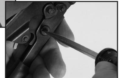
3. Adjust clamp tool jaws by rotating the eccentric stud counter-clockwise until jaws contact gauge. Re-tighten the locking nut.
