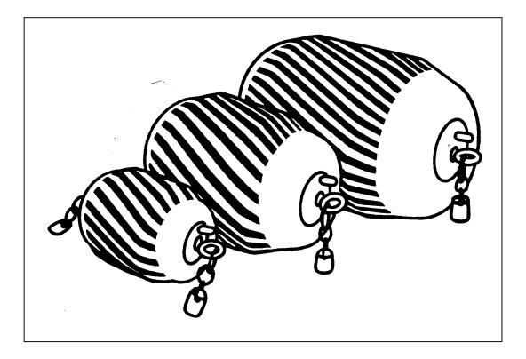
The Jet-Ball<sup>®</sup> pipeline cleaning ball uses the force of water to spin and scrub pipes clean. The ball's spiral ribs create the spin, while eyebolts on each end of the ball allow it to move in either direction through pipe. The following instructions describe how to install and operate your cleaning ball.
