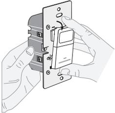
Push down tabs per diagram, one at a time and rotate forward to release
