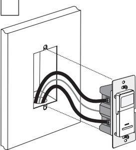
**NOTE:** Dress wires with a bend as shown in diagram in order to relieve stress when mounting device.
