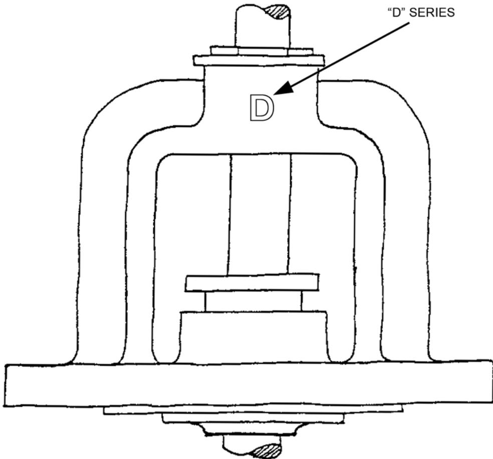
The “D” series valves are identified by the raised letter “D” cast into the bonnet as shown above.
