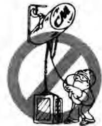
Do not operate with hoist head resting against any object. Lift the load gently. Do not jerk it.
