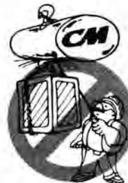
Do not use load chain as a sling. Such usage damages the chain and make the lift limit devices ineffective.
